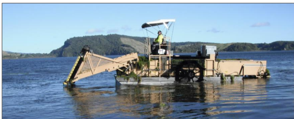
Figure 4.6: A lake macrophyte harvester in operation on Lake Rotoehu (source: www.lakeweeds.co.nz ).
