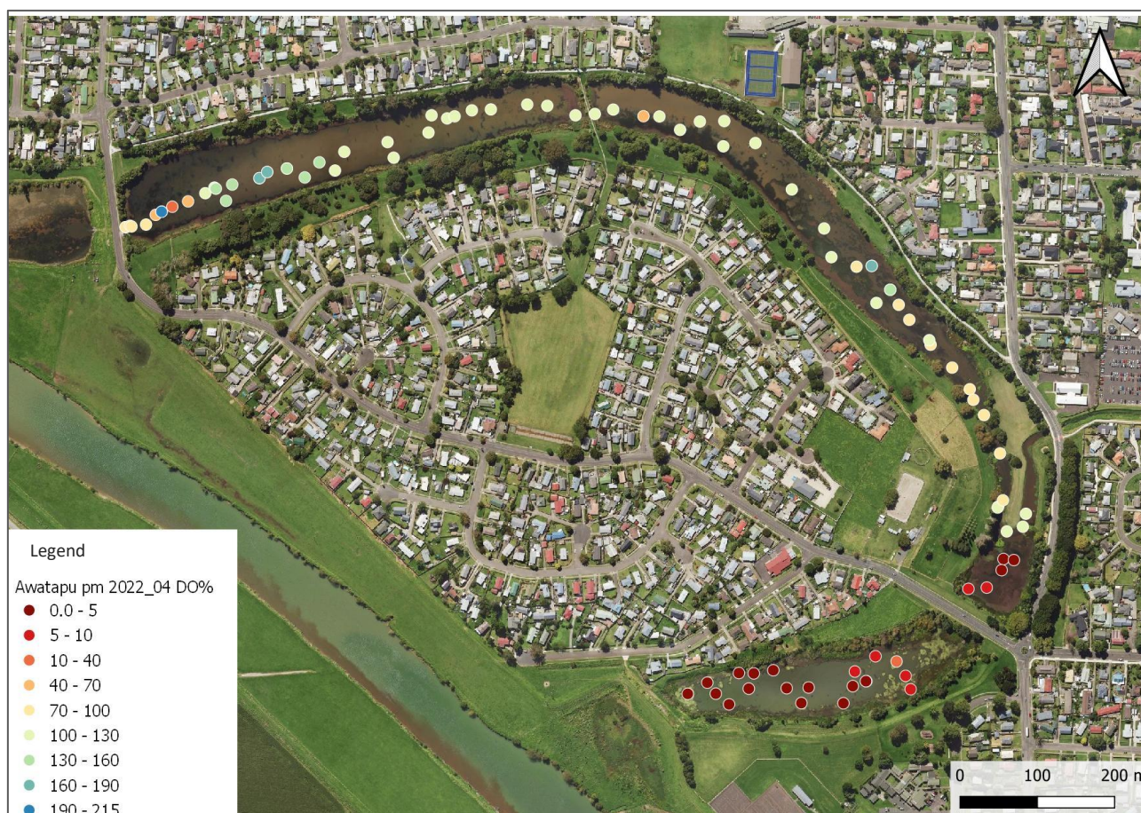
Figure 3.16: Spatial variation of dissolved oxygen saturation (%) in Awatapu Lagoon during late afternoon on 11 April 2022. High DO saturation in the western lagoon is associated with the photosynthesis of hornwort mats in this part of the lagoon. Very low DO saturation in the southern lagoon and near the Wainui Te Whara delta is consistent with decomposition of macrophyte organic matter in this area.
