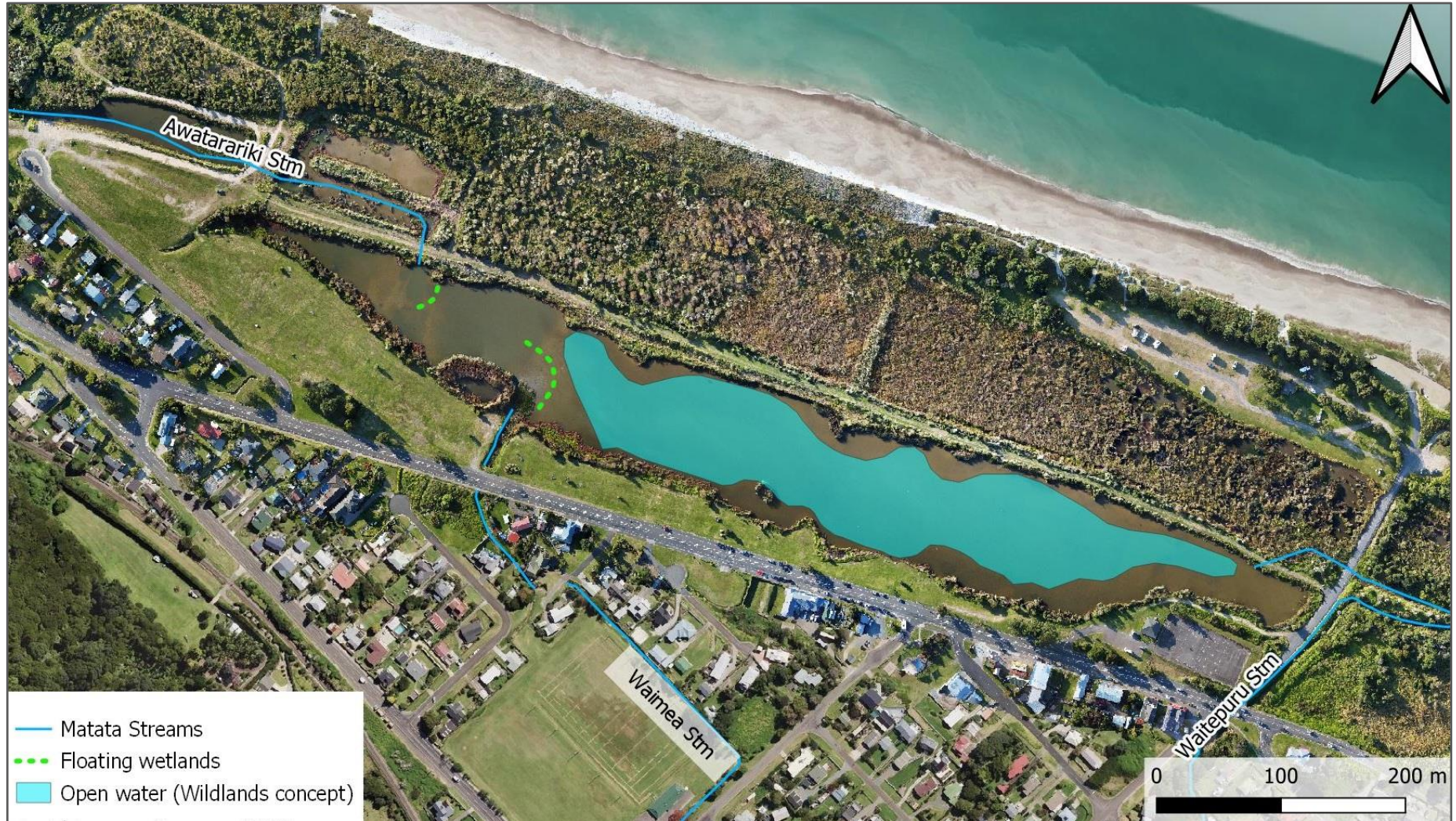
Figure 4.1: Western Matatā Lagoon showing approximate extent of open-water in concept plans for remediation works, and possible locations for floating wetlands. White flowers of pampas are visible along the walkway and in the western end of Floodway Bay 2, indicating areas requiring plant best control. (Aerial image, May 2024).
