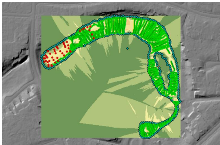
Figure 2.1: The three sets of depth points used to create a Digital Elevation Model for Lake Sullivan. Depth-sounder (green), lead-line (red), and water margin (blue).
