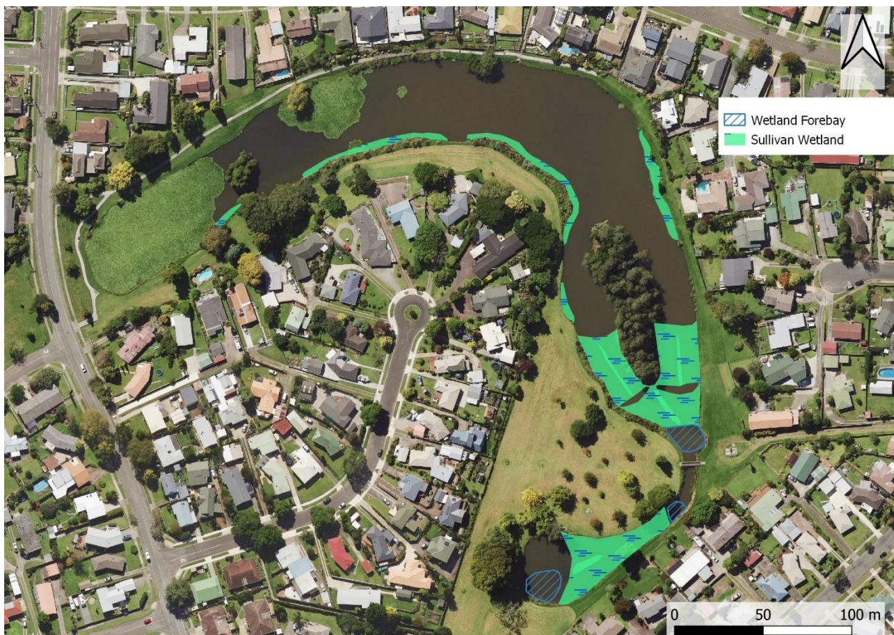
Figure 4.1: Potential layout for a treatment wetland and riparian wetlands in Sullivan Lake to improve water quality and provide biodiversity values.
